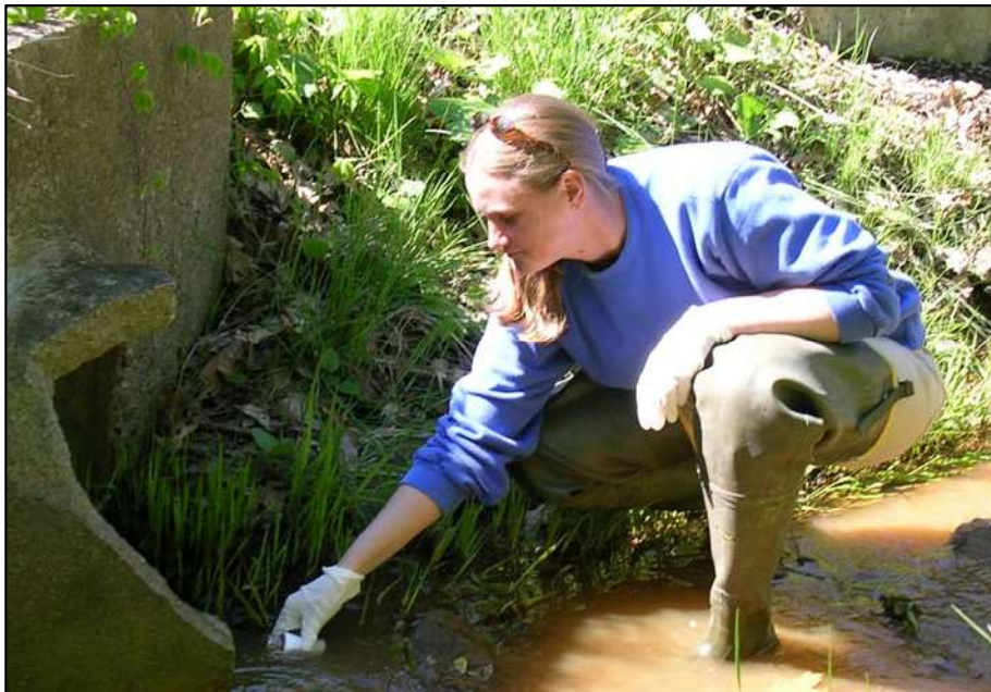
Figure 13: Taking a water sample at an MS4 outfall location during dry weather flow.
